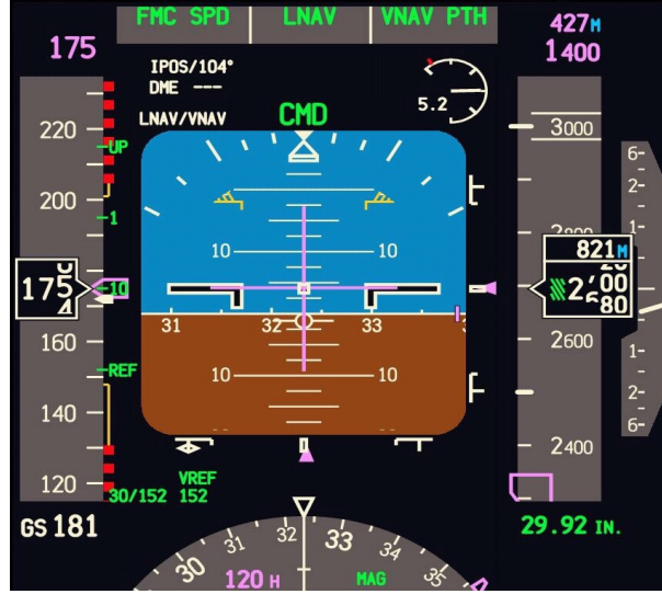
Figure 2.3: Primary Flight Display of a Boeing 737-800 [19].
